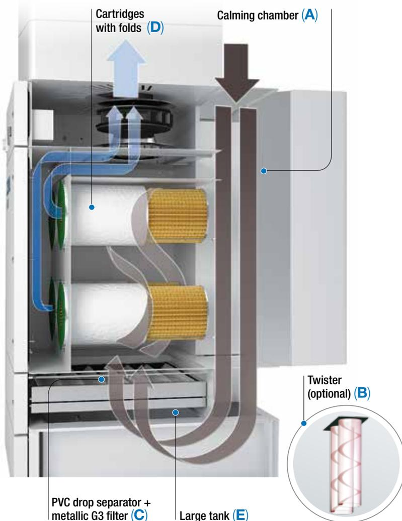
houses the filter elements, cartridges with folds (D), with a high filtration surface which withholds the finer impurities. These cartridges are covered by a highly absorbent, coalescent filter which also allows for an even distribution of the air flow over the entire cartridge. This filter has a filtration efficiency of F5, namely 40-60%, while cartridges have an efficiency of F9 about 95%.
